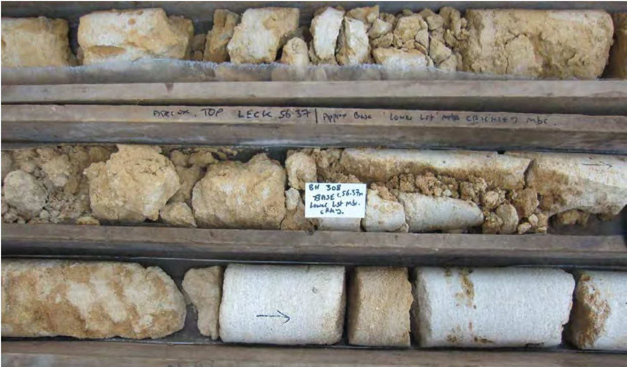
Figure 9 BH308. Middle run showing contact between top Leckhampton limestone (LECK) and approximate base of the 'lower limestone' unit of the Crickley Member (CRKY-BLPL) of the Birdlip Limestone Formation. Arrows indicate way-up with top of core on right hand side. Core is approx. 100mm (4") diameter.
