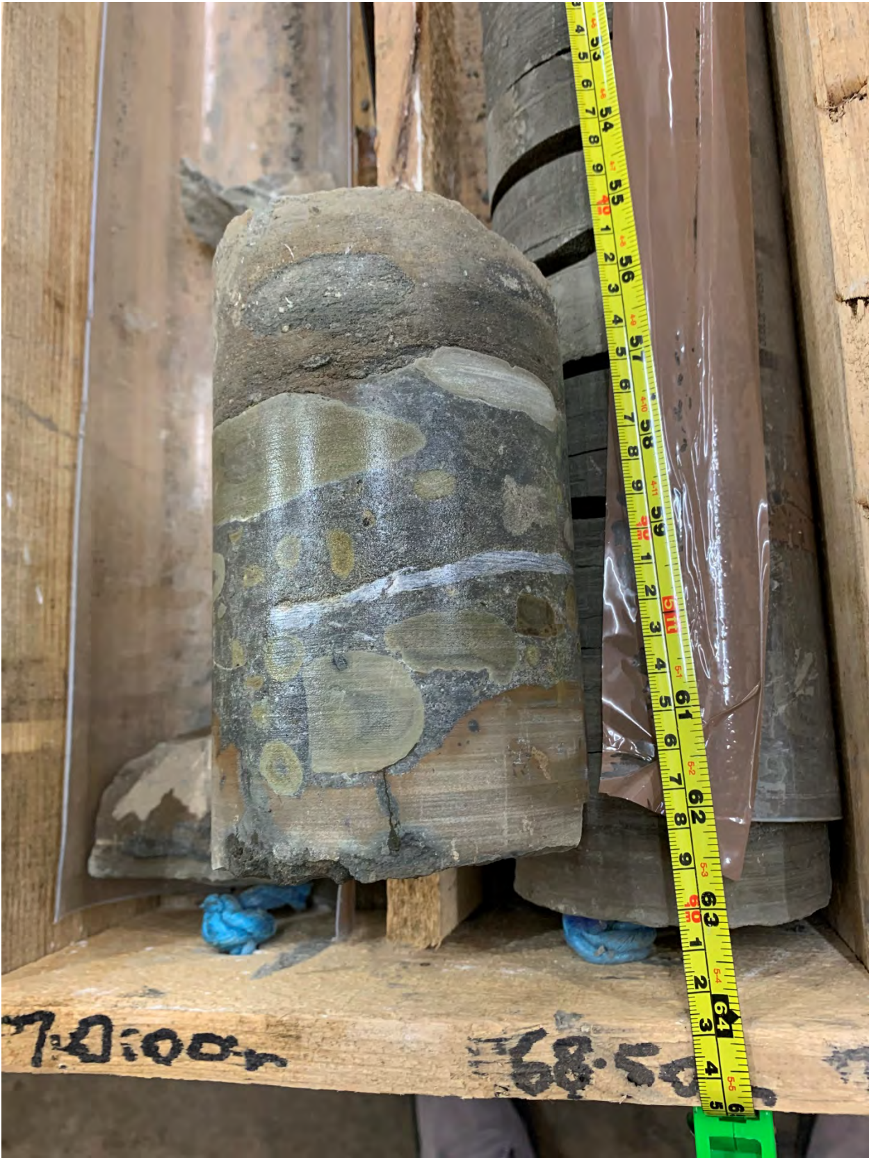
Figure 3 BH224 at 70.0m. Marlstone Rock (MRB). Very strong to strong grey limestone with distinctive rounded sideritic siltstone pebbles at base.
