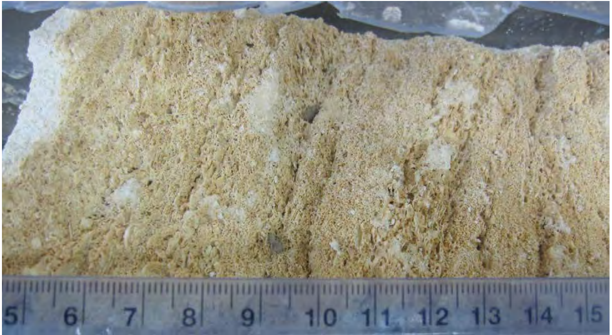
Figure 14 BH308. Close up photo of the typically light brown shell-detrital 'Fiddlers Elbow' limestone (packstone) at the base of the Cleeve Cloud Member (CLCL-BLPL). Scale bar is in cm.
