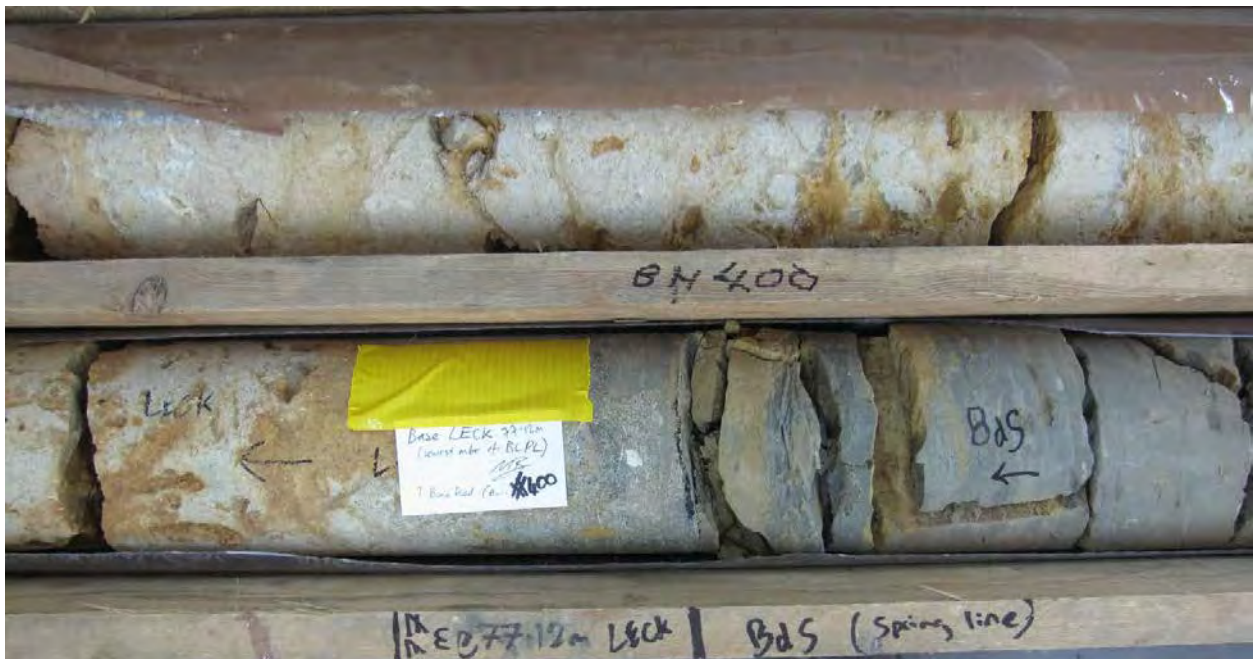
Figure 8 BH400. Lower run showing contact between 'strong', grey, limestone at base of Leckhampton Member (LECK) and weaker dark grey interlaminated mudstone and fine sands
