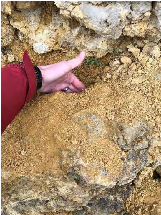
Photograph 61: Photograph of face-parallel joints 80dip/359dip direction. Open sub-vertical joint max 30mm. Joints pass down and along bedding planes. Photo looking 90°.
