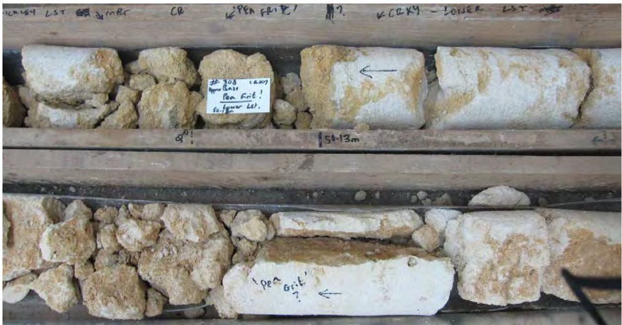
Figure 11 BH308. Approximate boundary (placed at 50.13m) between approximate base of rubbly 'Pea Grit' limestone and top of more competent/strong 'lower limestone' unit of Crickley Member (CRKY-BLPL). Arrow shows way-up/points to top of core. Lower boundary of 'Pea Grit' taken as were the distinctive oncoidal-rich limestone beds become more common than the strong white micrite limestone.
