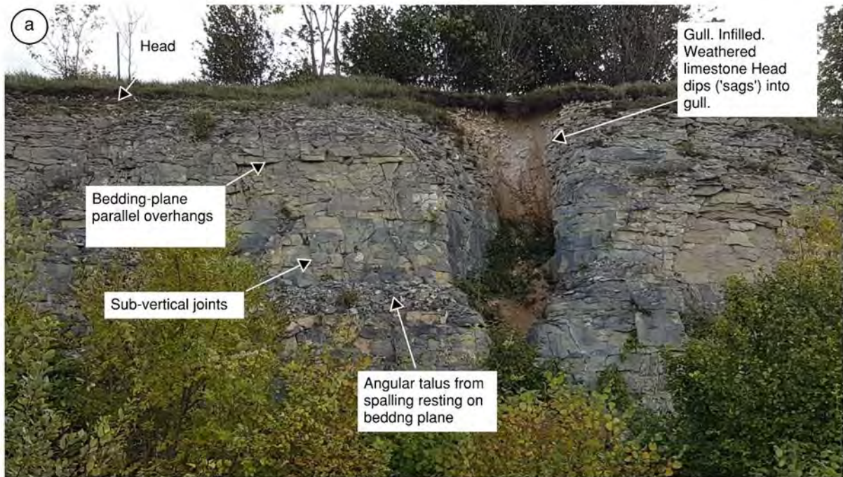
Photograph 73: Evidence of gulls from site walk over 10 th October 2019. a) Crickley Hill, north [392966, 216333], bi) Crickley Hill, north [392835, 216307], bii) close-up of part of bi) and c) Crickley Hill, south [392961, 215983]
