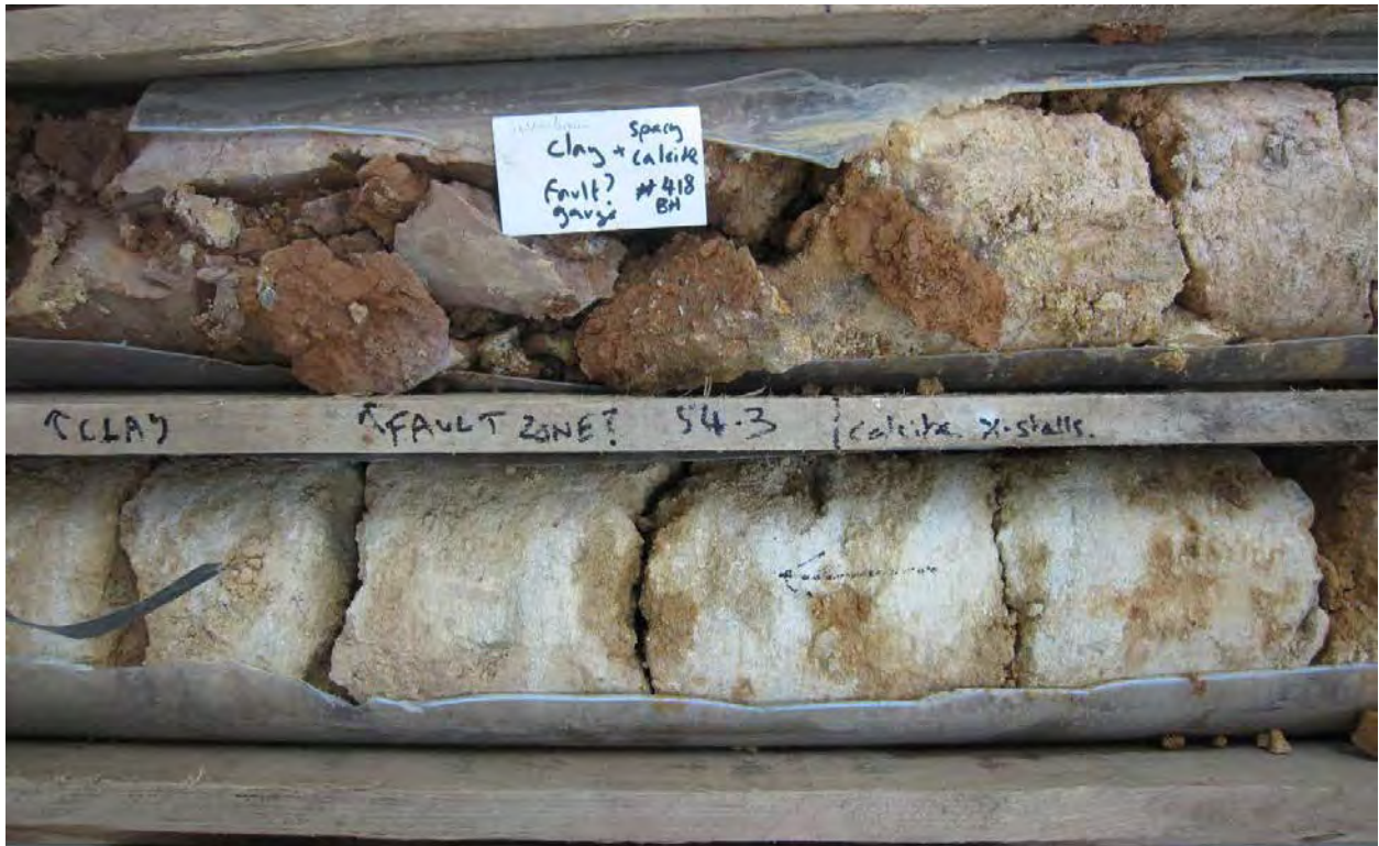
Figure 10 BH418 at 54.3m. Upper run shows red-brown stiff clay gauge with rhomboidal (probably calcite) crystals formed in wall rock. Interpreted by BGS as possible fault zone or in-washed palaeo-karst feature. Lower run is ferruginous orange 'strong' limestone typical of the upper part of Leckhampton Member (LECK-BLPL).
