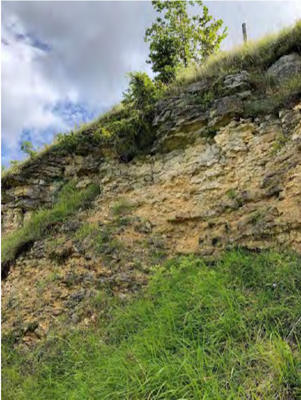
Photograph 50: IMG_3410. Photograph of an exposure of IO on the northern side of Crickley Hill. The exposure shows the rubbly nature of the pea grit (pale orangish brown surface) at the base of the exposure. Compared to the overhanging bedded limestone (IO) above. Photo looking 150°.
