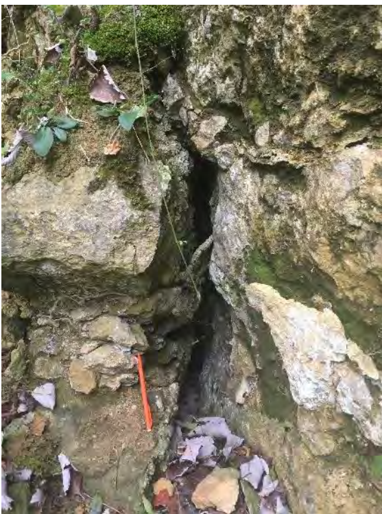
Photograph 65: Photograph of large sub-vertical joints and deep voids. Overhanging limestone (IO) beds. and some dissolution holes. Photo looking 300°.
