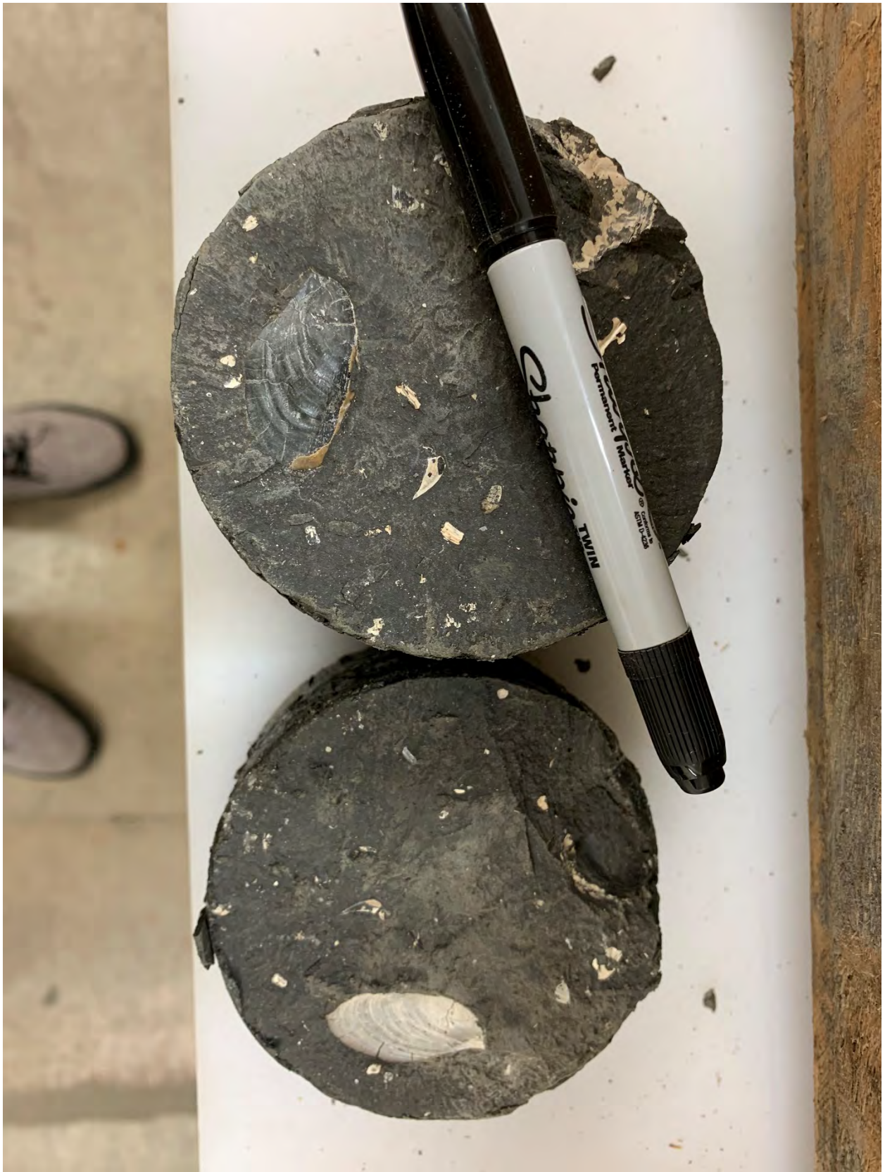
Figure 5 Typical Whitby Mudstone Formation (WHM) weak laminated dark grey mudstone with bivalve and ammonite (pink aragonite) fossil content.
