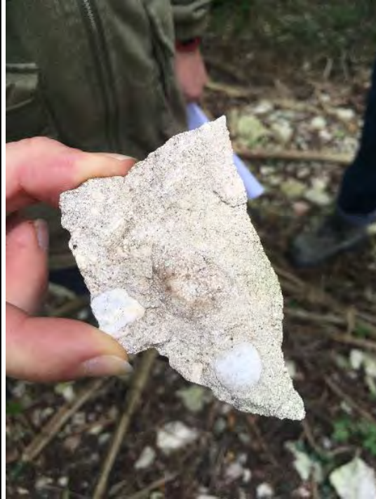
Photograph 4: IMG_9529. Photograph of sample of Inferior Oolite. Noted to be primarily ooidal with whole shelly fossils. Photo looking 200°.
