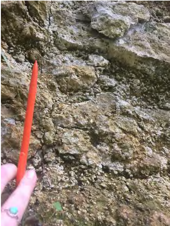
Photograph 65: Photograph of large sub-vertical joints and deep voids. Overhanging limestone (IO) beds. and some dissolution holes. Photo looking 300°.
