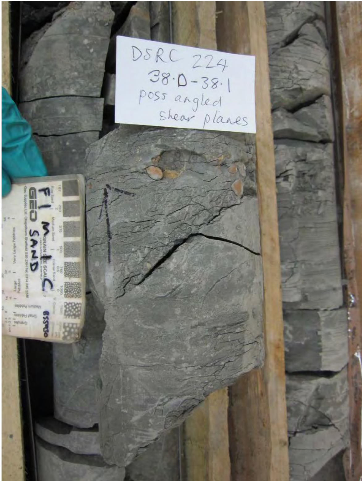
Figure 4 BH DSRC224: Possible shear zone in Whitby Mudstone Formation mudstone at 38.0-38.1m. Note brown small gravel-sized litho-relicts of ferruginous siltstone in upper half of core and dark grey laminated mudstone in lower half.
