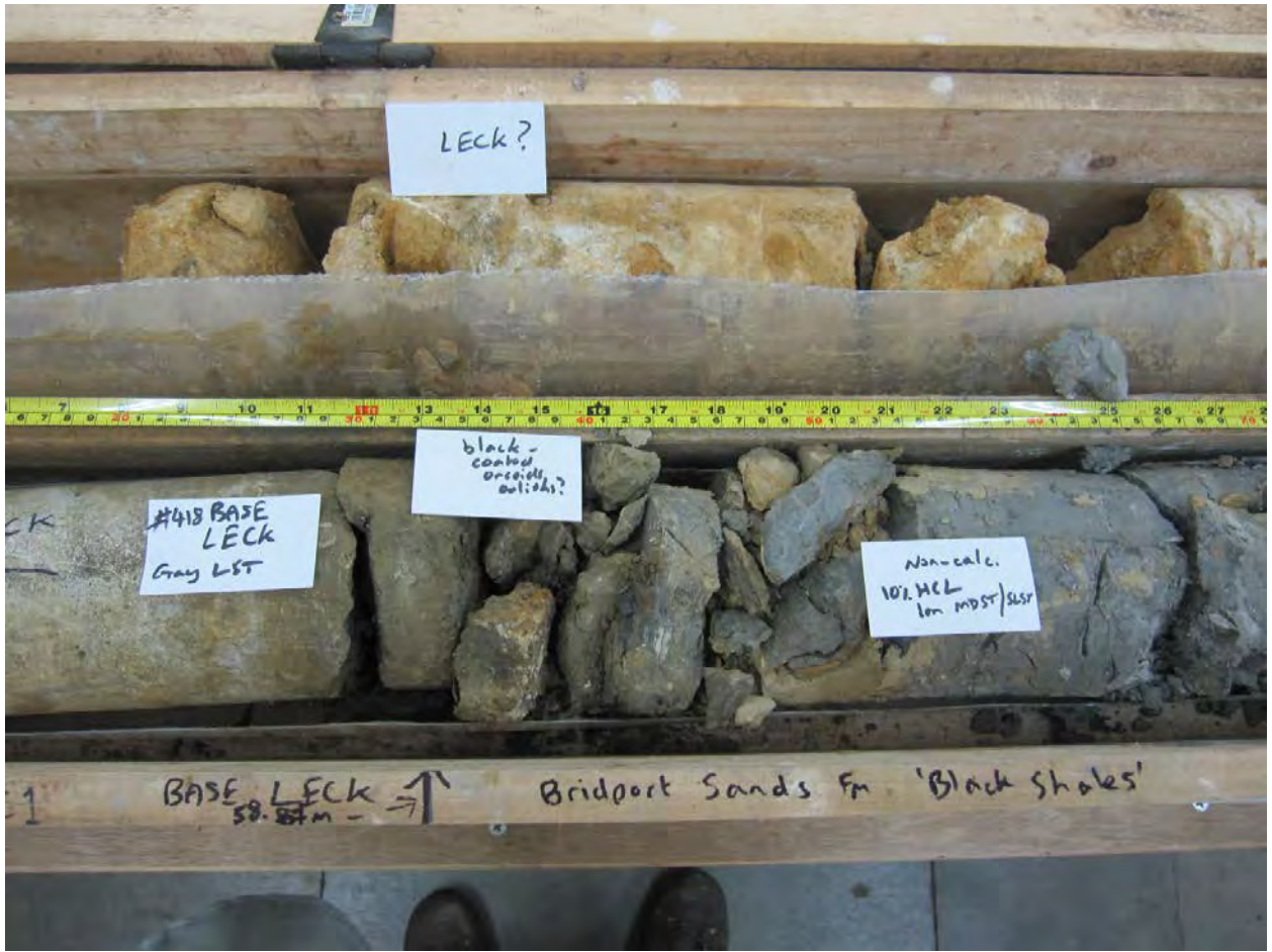
Figure 7 BH418: Lower run showing sharp contact between 'very strong' grey limestone at base of Leckhampton Member (LECK-BLPL) with underlying 'weak' dark grey laminated 'black shale' mudstone unit at top of Bridport Sands Formation.
