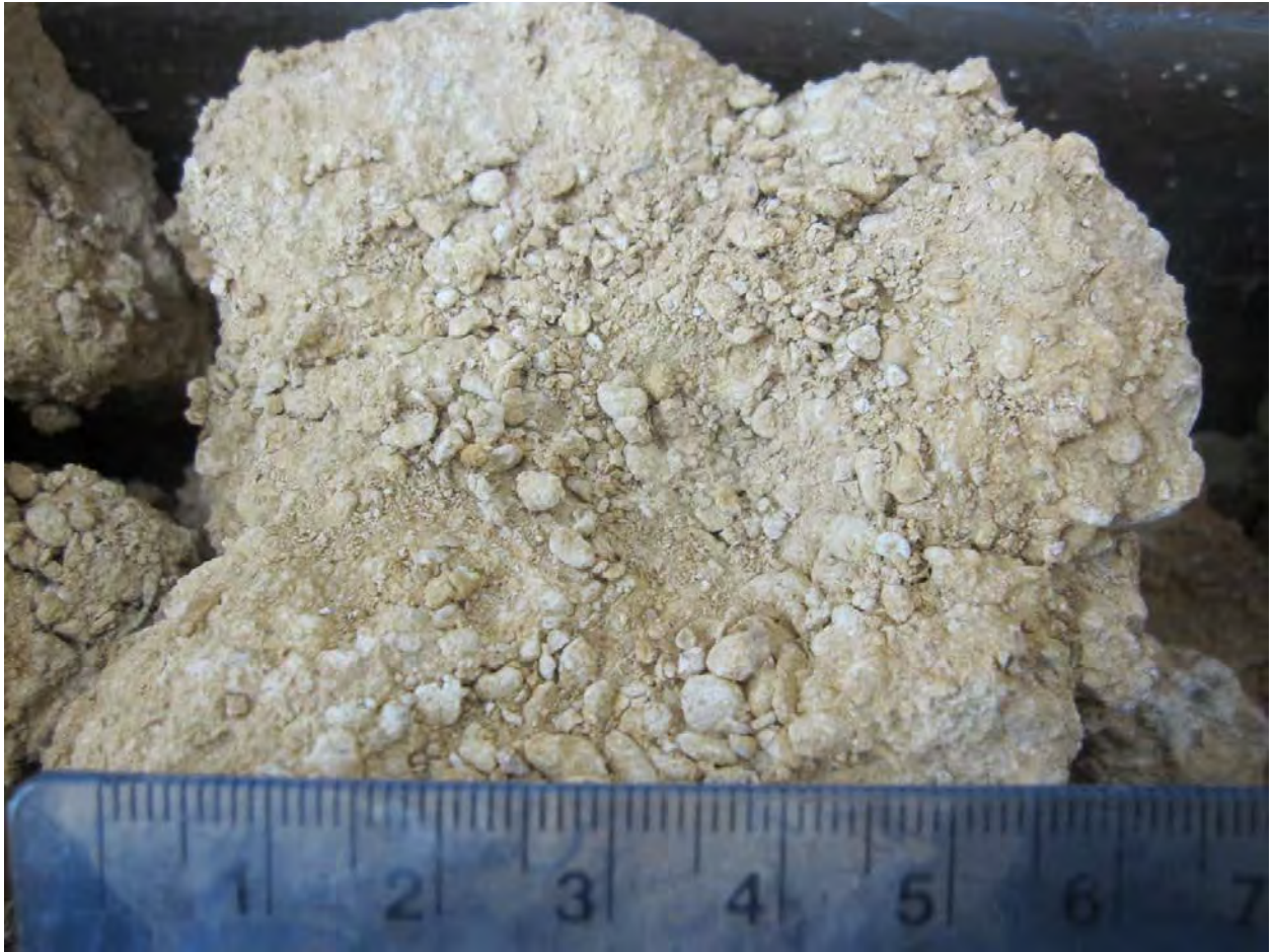
Figure 12 BH308. Close up photo of typical 'Pea Grit' unit in upper part of Crockley Member (CRKY); moderately weak limestone rock, packed full of medium to coarse sand-sized disk-shaped oncoids (1-5mm dia.), rubbly rock mass, loosely packed with large voids (indicated by core loss and confirmed by geophysical logs), variable strength, poorly cemented. Scale is in cm.
