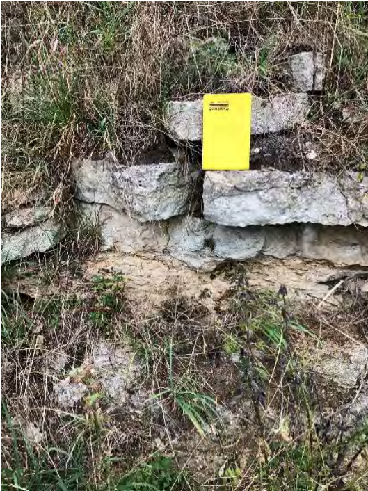
Photograph 15: IMG_3264. Photograph of bedded limestone (interpreted to be GOG). Circa 200mm spacing between beds. Bedding structure 12/162 SE. Photo looking 040°.
