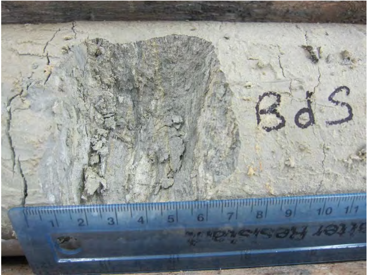
Figure 6 BH400. Close-up photo of typical Bridport Sand Formation (BDS) with grey fine-sand with subordinate white wispy sand laminae. Very weak to weak rock.
