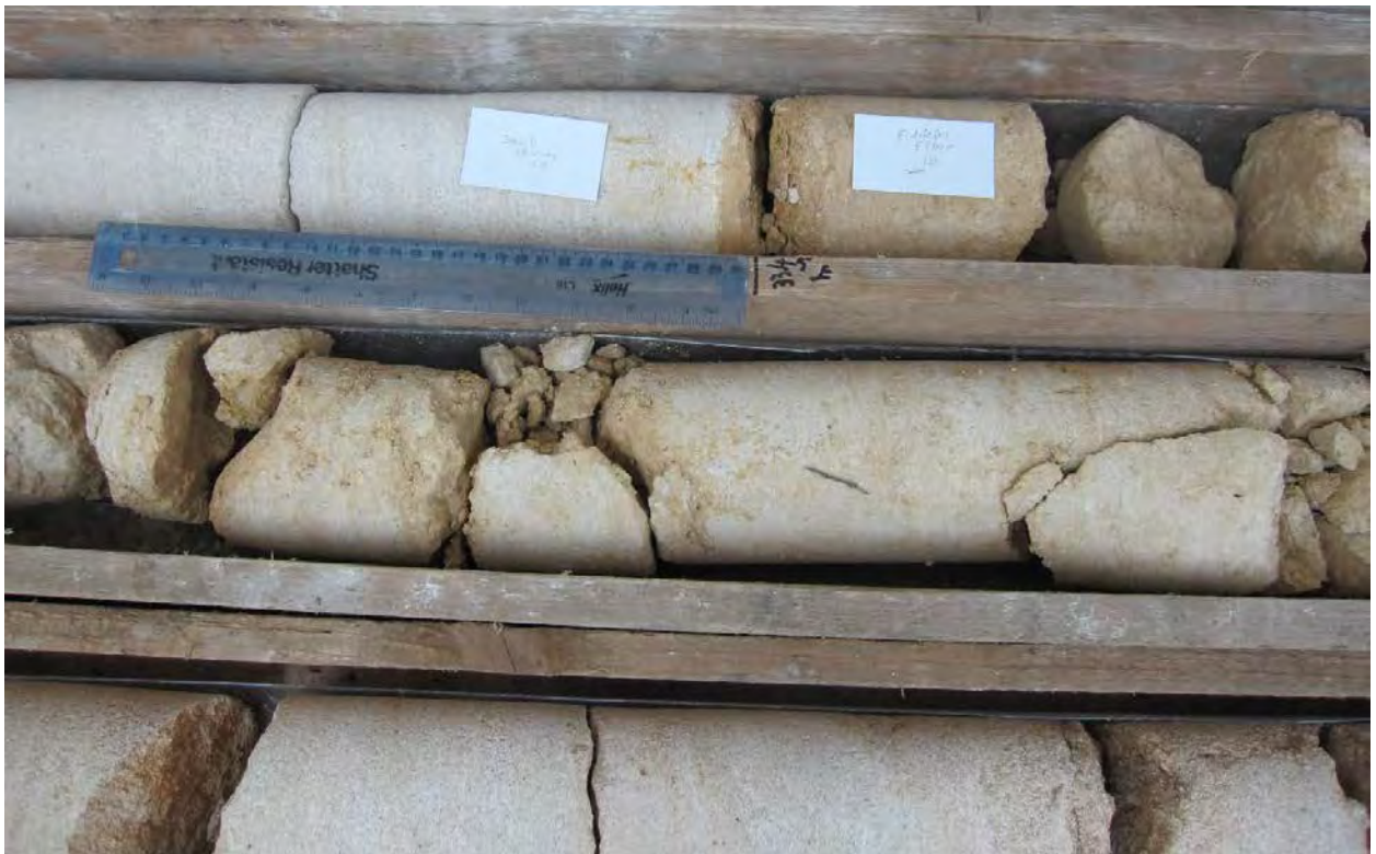
Figure 15 BH308. Upper run is gradational boundary between light brown shell-detrital 'Fiddler's Elbow' limestone and overlying white, ooidal, 'Devil's Chimney Oolite' (grainstone) in the upper part of the Cleeve Cloud Member at the top of the Birdlip Limestone Formation. Lower two runs are typical Devil's Chimney Oolite'.
