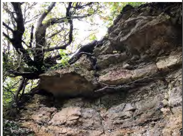
Photograph 66: Photograph of large sub-vertical joints and deep voids. Overhanging limestone (IO) beds. and some dissolution holes. Photo looking 300°.
