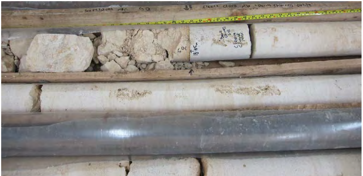
Figure 16 BH308. Sharp boundary (at 18.85m) between 'Devil's Chimney Oolite' at upper Cleeve Cloud Member and the cream limestones (grainstone) of the Scottsquare Member at top of Birdlip Limestone Formation. 'Sq' at 18.85m marks a weaker marly layer coincident with a gamma peak in the downhole geophysical logs. Diagnostic clusters of Brachiopods can be seen in a freshly broken surface on the left hand side at around 18.5m. Middle and lower runs are typical Scottsquare Limestone.
